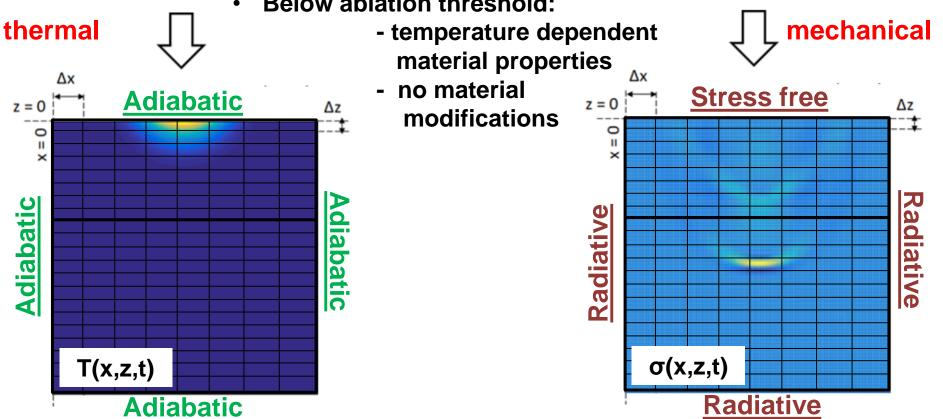
Irradiation by laser pulses, below ablation threshold Nd:YAG, 7 ns,  $\sim 0.1 \text{ J}$
