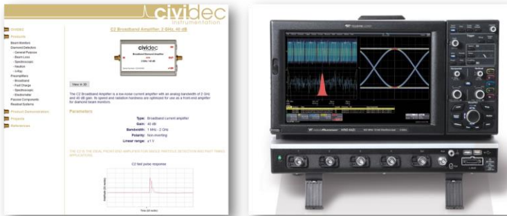
WaveRunner 625Z1 2.5 GHz, 20 GS/s, 4ch, 16 Mpts/Ch DSO with 12.1" WXGA Color Display, 50 ohm and 1 Mohm Input, 40 GS/s and 32 Mpts/Ch in interleaved mode.
