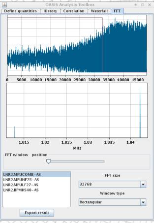
Baseband content: ~3.5KHz noise (most likely, power supply ripple)
