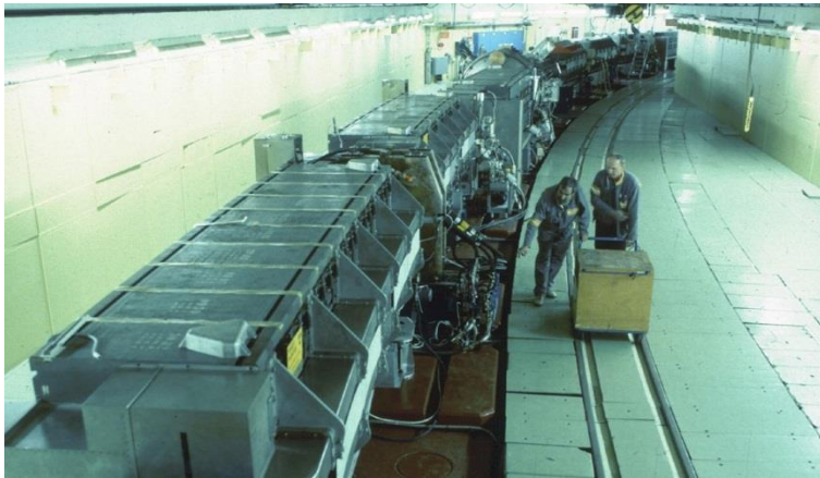
200-m diameter ring, weight of magnets 3,800 tons
