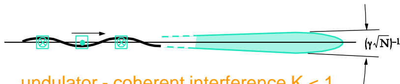
undulator - coherent interference K < 1
