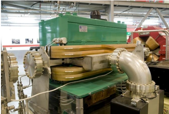
Sextupole magnets to focus off-energy electrons (mainly)
