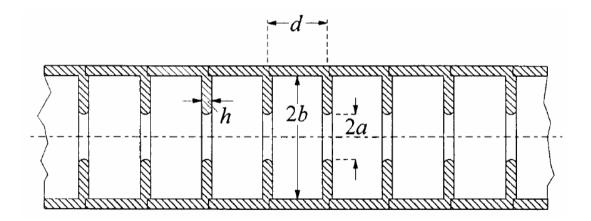
Assuming that the cavities are operated in the  $2\pi/3$  mode with a phase velocity  $\beta_z = 1$  and a supplied power of 35 MW, what is the total accelerating voltage and energy gain per metre for a SLAC structure of length l = 3 m.?
