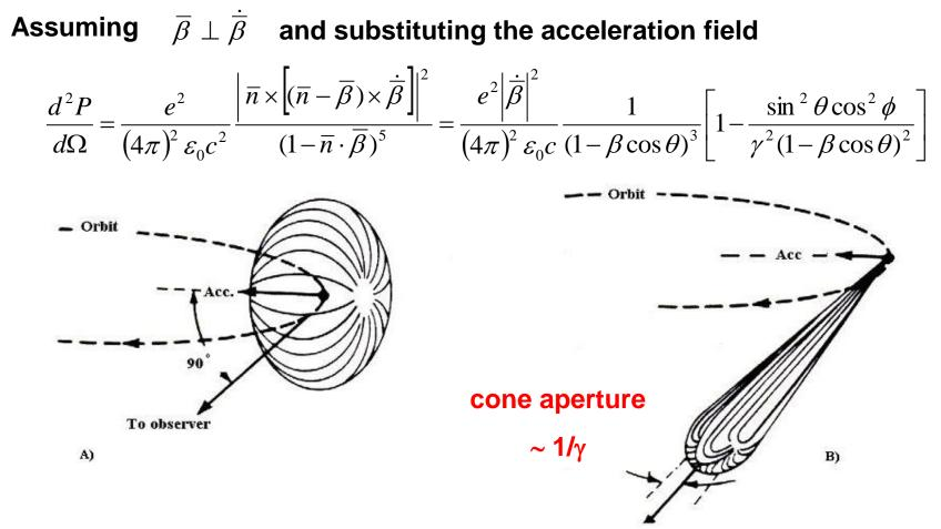
When the electron velocity approaches the speed of light the emission pattern is sharply collimated forward
