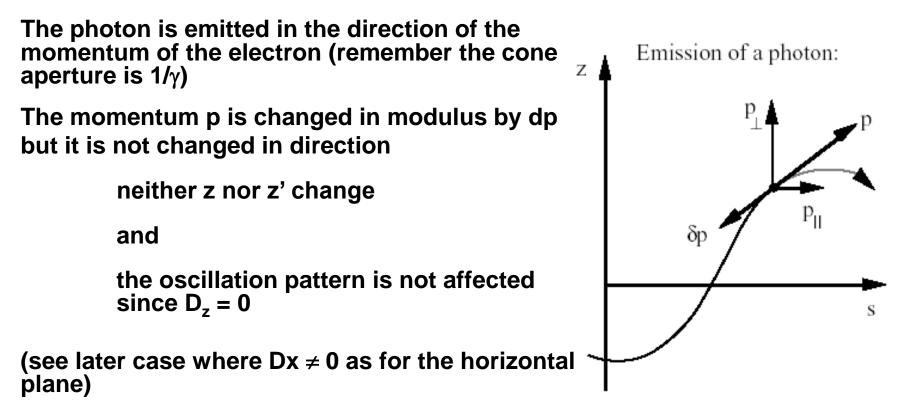
Therefore the Courant-Snyder invariant does not change as result of the emission of a photon
