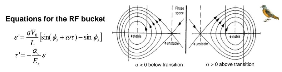
Aide-memoire for stable motion: above transition the head goes up in energy, below transition the head goes down in energy
