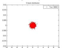
After 50 synchrotron periods (~2 radiation damping time) the longitudinal phase space distribution has almost reached the equilibrium and is matched to the RF bucket
