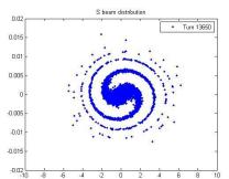
After 50 synchrotron periods the longitudinal phase space distribution is completely filamented (decoherence).
