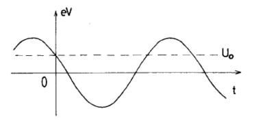
A particle in an RF cavity changes energy according to the phase of the RF field found in the cavity
