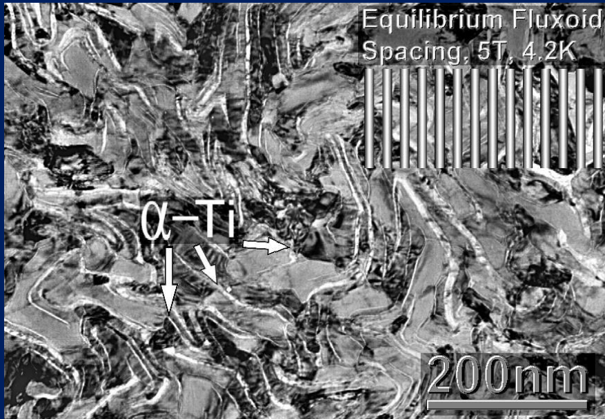
Microstructure of Nb-Ti
