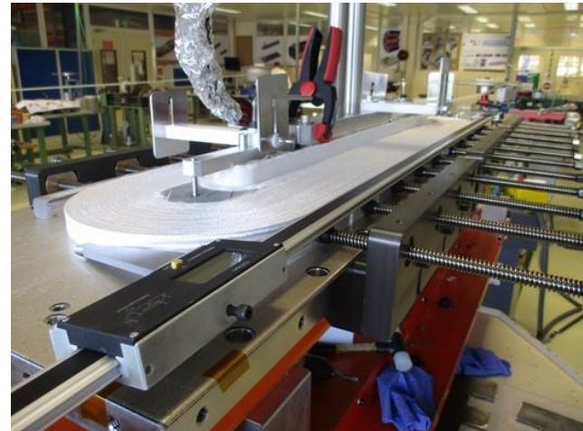
First ERMC coil winding
