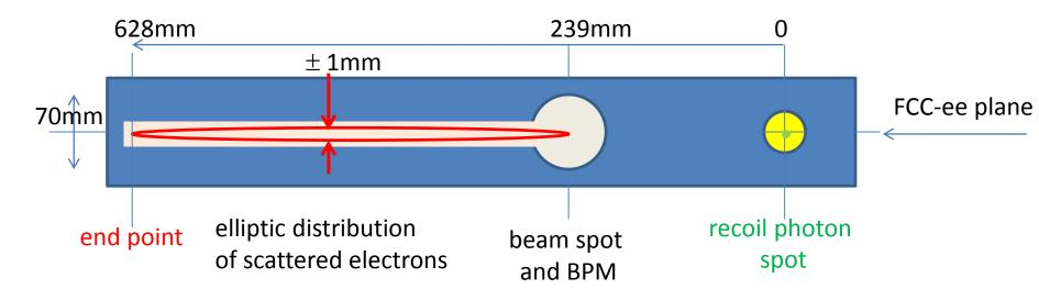
The end point moves by 0.24 microns over 628 mm (0.3 10<sup>-6</sup>) These relative movements are perhaps visible using a silicon pixel array. The absolute measurement in the underground conditions seems difficult.
