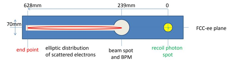
polarimeter-spectrometer situated 100m from end of dipole.
