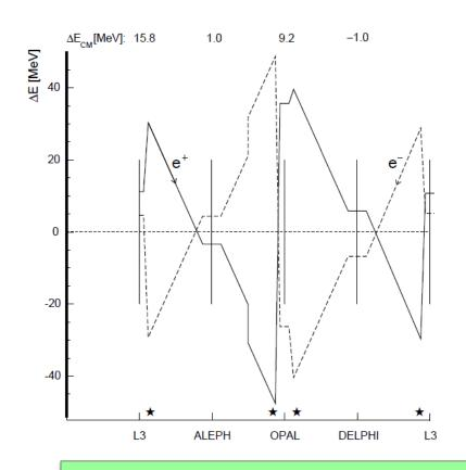
Errors arise due to cavity misalignments primarily:
