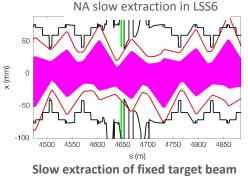
at 400GeV, incl. extraction bump purple : raw beam envelope red: beam envelope + tolerance
