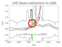
Fast extraction to LHC Crab-cavity in beam does not yield enough aperture for extracted beam
