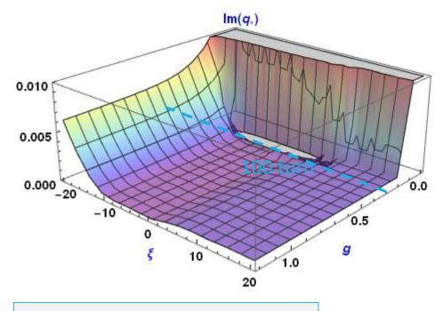
Damper gain: g = damping rate /  $\omega_s$ Growth rate: Im q = rate /  $\omega_s$
