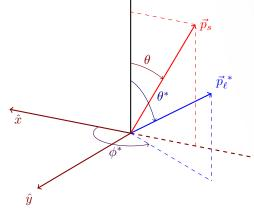
$$\frac{1}{N} \frac{dN}{d\Omega d\Omega^*} = \frac{1}{(4\pi)^2} \left[ \frac{3}{4} \left| A_{1,\frac{1}{2}} \right|^2 (1 + P\cos\theta) \left( 1 + \cos\theta^* \right)^2 \right] F_L$$
