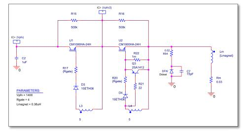
Above: PSpice Model for Series Switch Architecture, P. Van Trappen: Further information: <u>New design concepts for suppressing erratic triggering</u> of solid state switch stacks (P. Van Trappen et al, FCCWeek 2017)
