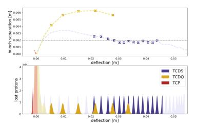
Load on and bunch separation at extraction absorber and primary collimator for 1 us risetime (shaded areas: by absorbers not intercepted p+)
