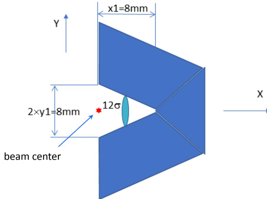
Schematic view of the cross-section of the right half of the TSCV collimator acting on protons with  $\delta_p < 0$ . The red star shows the beam center while the teal ellipse shows the  $12\sigma$  envelope for  $\delta_p = -0.0015$ .
