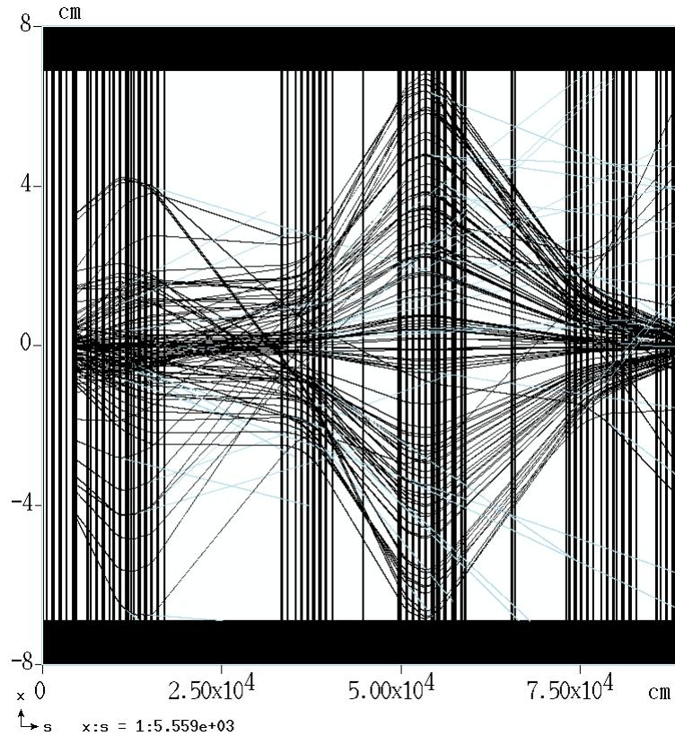
Proton trajectories in horizontal (left) and vertical (right) plane. MARS notations differ from conventional  $x \leftrightarrow y$
