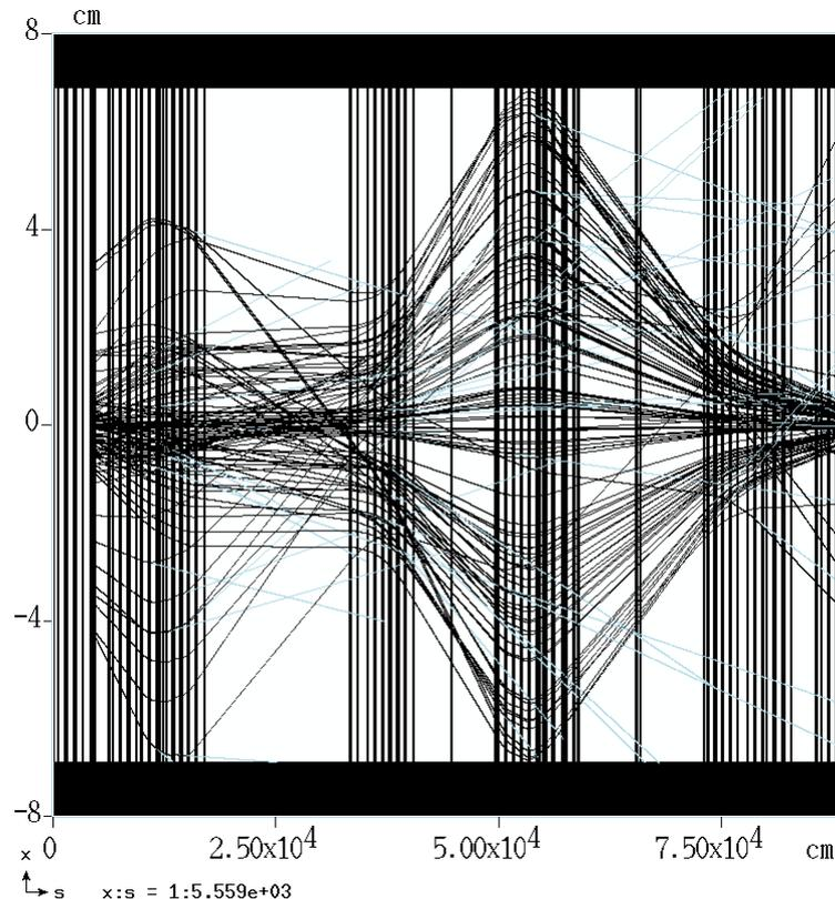
Proton trajectories in horizontal (left) and vertical (right) plane. MARS notations differ from conventional  $x \leftrightarrow y$
