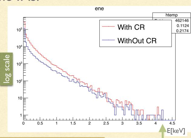
The maximum energy of these photons has been reduced due to weaker bending magnets
