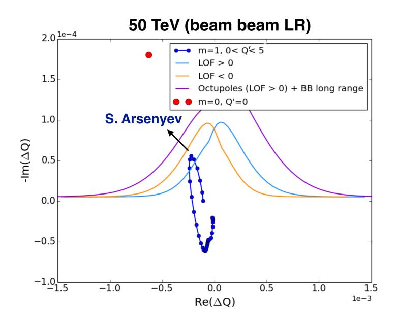
■ Tune spread from bb LR and positive octupoles adds up  $\rightarrow$  larger stability but smaller DA: 5.8  $\sigma$  instead of ~7  $\sigma$  as in case of negative octupole polarity
