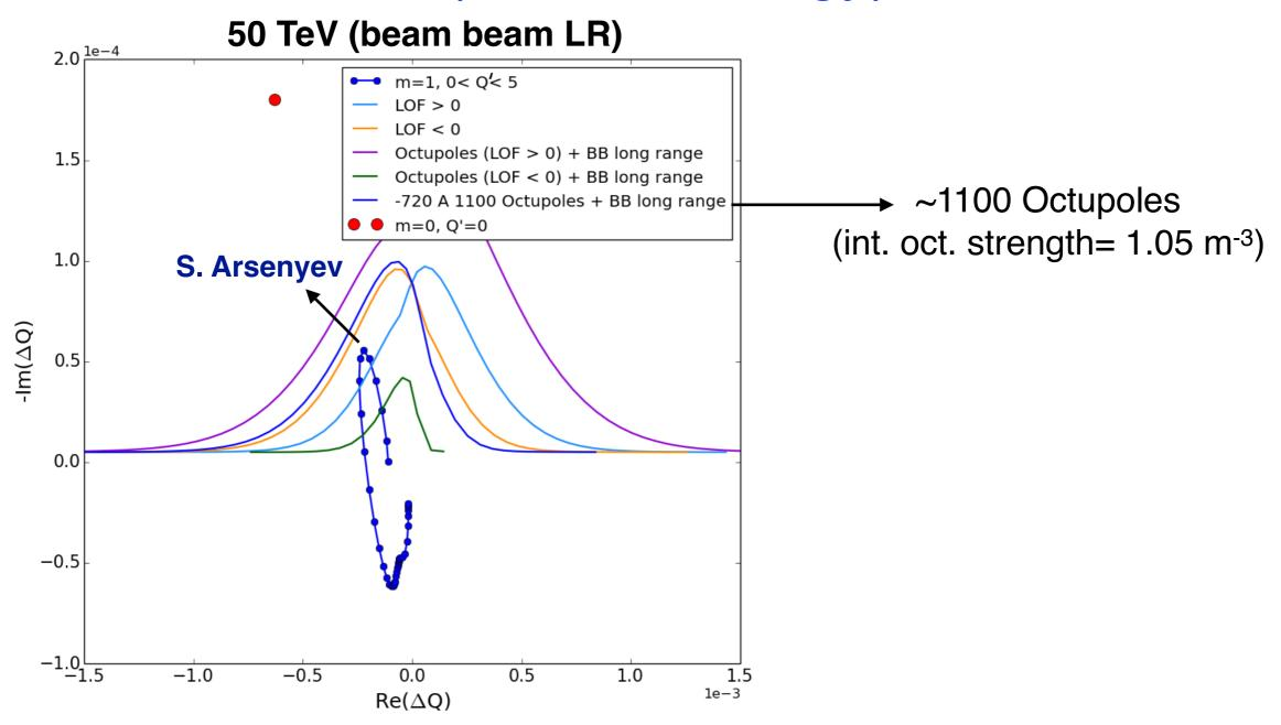
■ With negative octupoles polarity an int. oct. strength= 1.05 m<sup>-3</sup> is needed to compensate reduction due to bb long range  $\rightarrow$  DA ~8.5  $\sigma$
