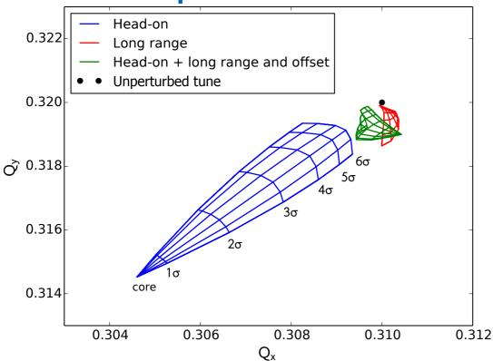
Detuning with amplitude (Octupoles magnets, machine non-linearities)
