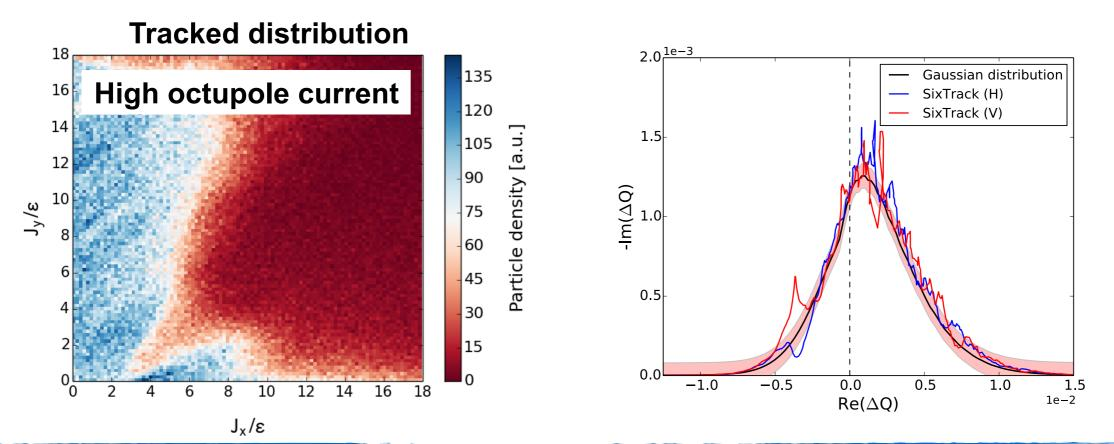
In presence of diffusive mechanisms and/or reduced dynamic aperture expected Landau damping may be reduced → evaluate impact of Dynamic Aperture [2]
