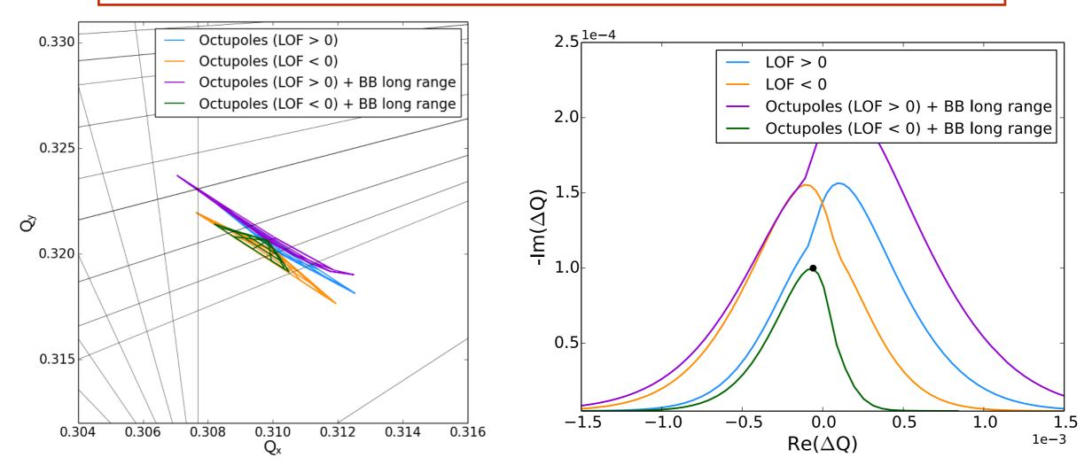
■ With negative octupole polarity and BB long range interactions, the stability is strongly reduced → the coherent impedance mode is not Landau damped
