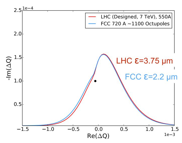
Considering the maximum FCC octupole strength and maximum current ~720 A ~1150 octupoles are needed to reproduce LHC stability (£=3.75 µm)
