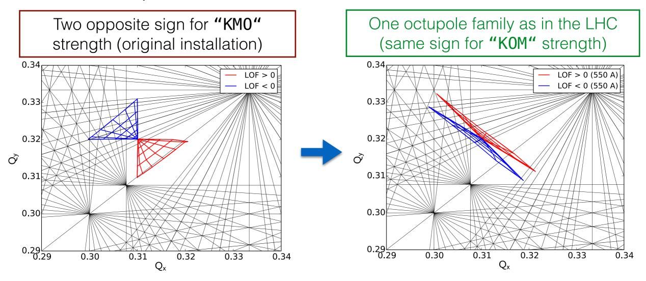
The original installation of the Landau octupoles was including opposite sign for "KM0" strength (opposite octupole polarity)
