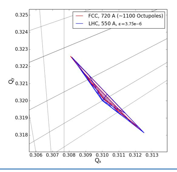
For FCC ~1100 octupoles are needed to reproduce LHC tune spread (ε=2.2 μm) powered with the maximum current of 720 A→ integrated strength ~ 1 [m<sup>-3</sup>] (~2.5 \* FCC<sub>strength</sub>)
