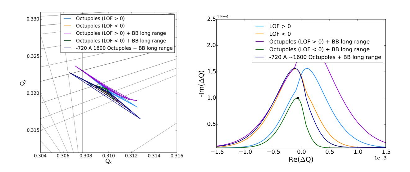
■ In order to recover the needed tune spread, an int. oct strength of ~1.5 m<sup>-3</sup> in case of negative octupole polarity and beam-beam long range interactions
