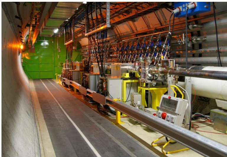
ADT kicker. The beam is kicked by electric field
