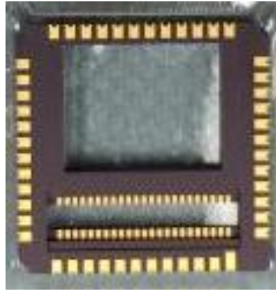
Same LCC with open center to minimize material in beam path
