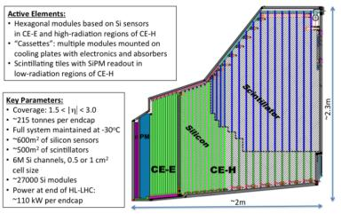
Electromagnetic calorimeter (CE-E): Si, Cu & CuW & Pb absorbers, 28 layers, 25 X<sub>0</sub> & ~1.3 $\lambda$  Hadronic calorimeter (CE-H): Si & scintillator, steel absorbers, 24 layers, ~8.5 $\lambda$
