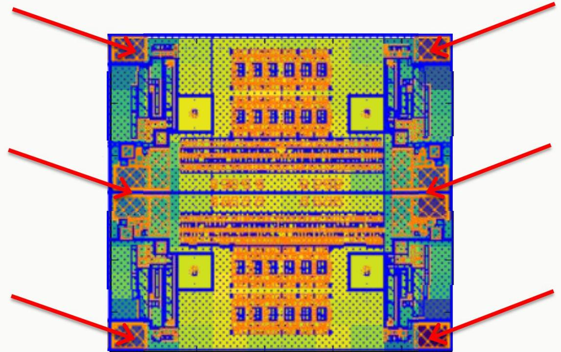
**Low efficiency "corners"** correlated with **large active areas** used for decoupling capacitors
