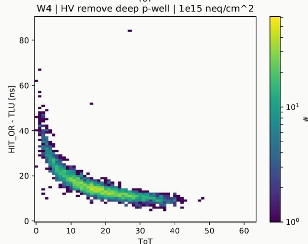
Distributions of "HIT\_OR signal - External trigger timestamp" in seed pixels from test beam (640 MHz sampling)
