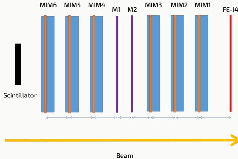
LF-MONOPIX (unirradiated and neutron-irradiated samples) exposed to MIPs at ELSA (2.5 GeV e-) and the H8 line of CERN's SPS (180 GeV pions)
