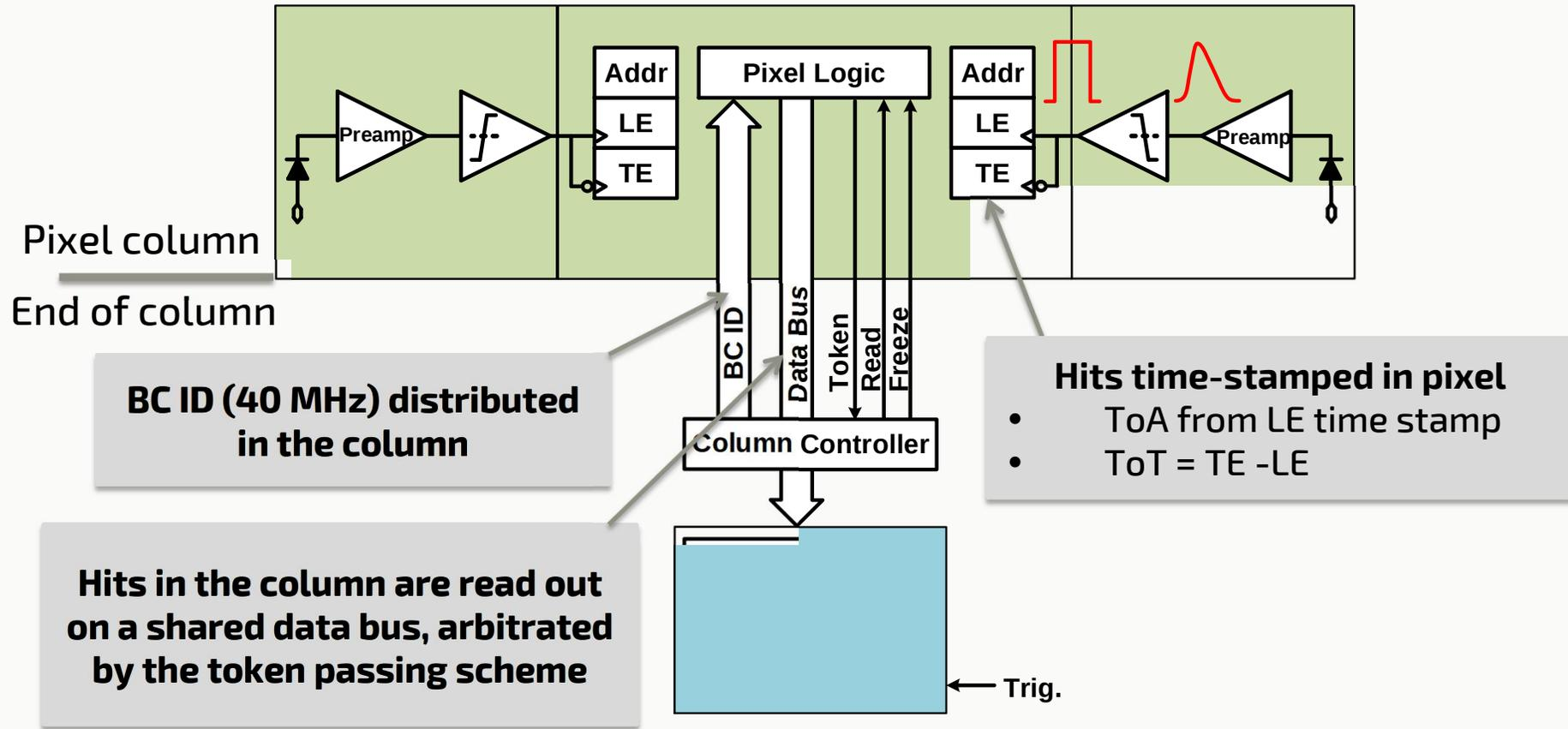
Column-drain has already proven to be capable to handle the hit rates of the current inner ATLAS pixel layers (FE-I3)
