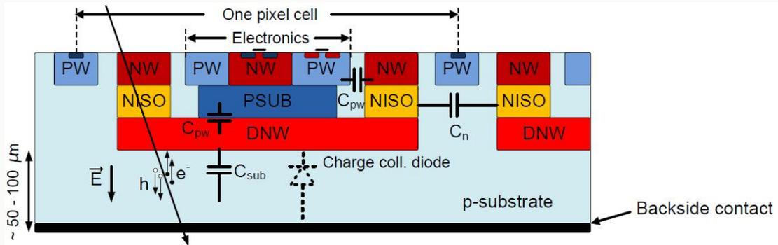
An increase in detector capacitance has implications on **timing** and **noise**
