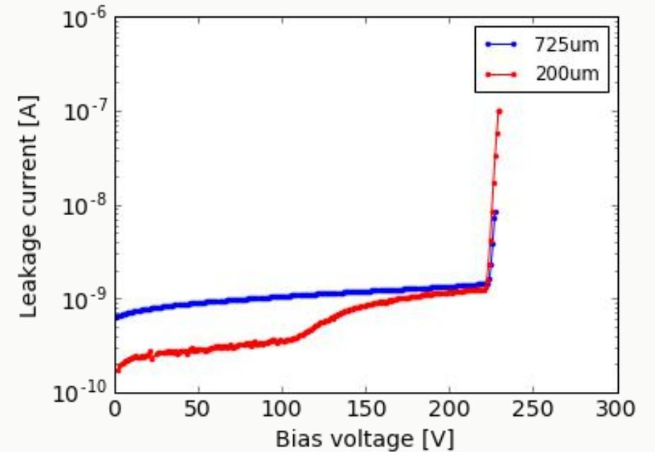
Reduction in leakage current after thinning and BS-process
