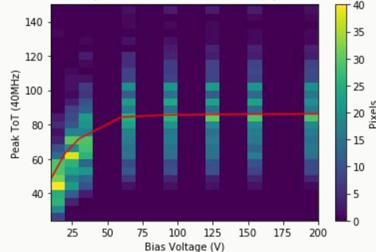
**200μm thick chip fully depleted at ~60V**
