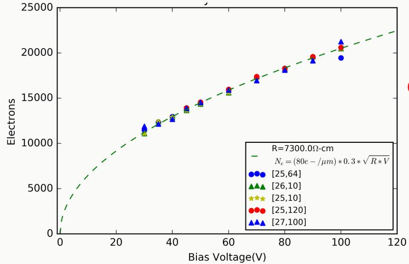
**Large collected charge (~10<sup>4</sup> e-) in a highly resistive (>2 kΩm-cm) substrate.**
