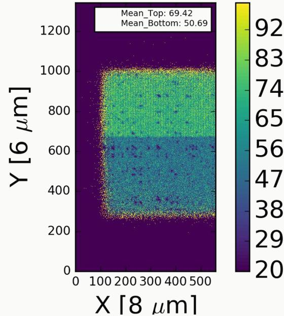
Large efficiency drop (30-50%) after  $1 \times 10^{15} \text{ n}_{\text{eq}}/\text{cm}^2$  neutron irradiation.
