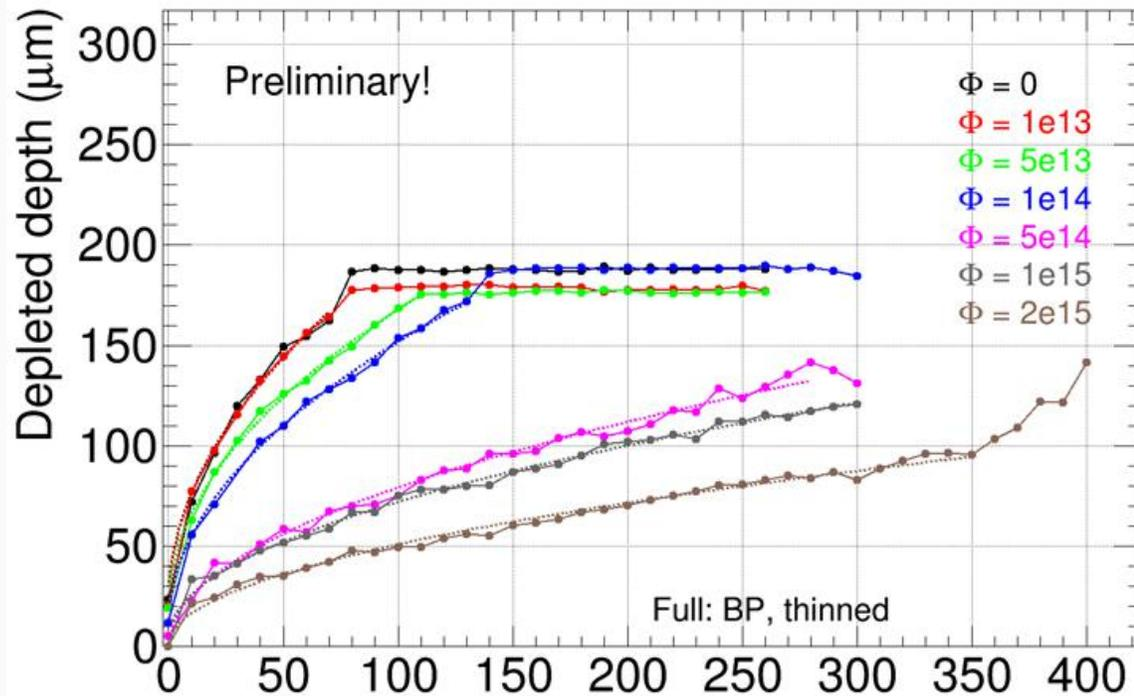
E-TCT measurement on LF test structures thinned to 200µm
