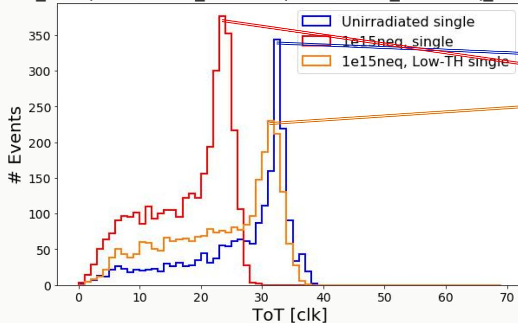
ToT vs Injection Rem\_DPW (Top) single-pixel.
