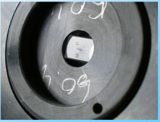
Dye laser power had to be reduced to avoid crystal damage
