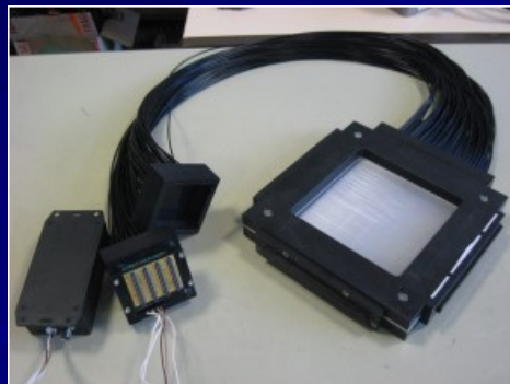
Scintillating-fibre Hodoscope + MA PMT Ray et al. IPN Lyon
