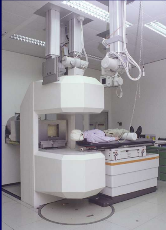
In-beam PET scanner at ^{12}\text{C} -therapy unit at GSI
