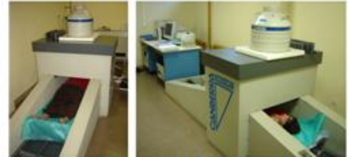
Figure 2. Measurement of whole-body and neck activity of radioactive iodine I-131 by using scanning-bed whole-body counter equipped with especially designed slit-collimator.
