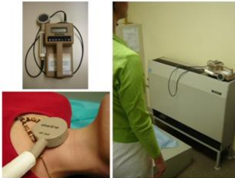
Figure 3. Measurement of neck surface dose rate and one-meter distance whole-body dose rate of radioactive iodine-131 by using beta-gamma exposure rate meter.
