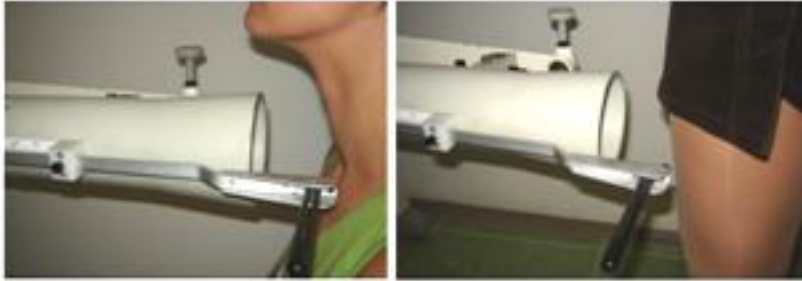
Figure 1. Measurement of radioactive iodine-131 activity in the neck and thigh (for background correction) by using conventional probe system.]
