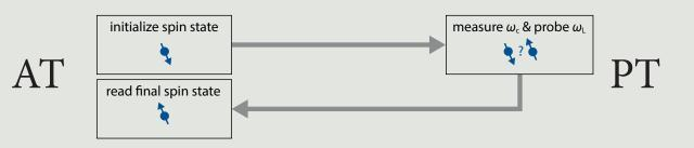
Application of a drive at the excitation frequency  $v_{rf}$  and simultaneous measurement of the cyclotron frequency  $v_c$  in the precision trap yields the ratio  $v_{rf}/v_c$  and probes the *g*-factor resonance (the spin-flip probability as a function of the ratio  $v_{rf}/v_c$ ).
