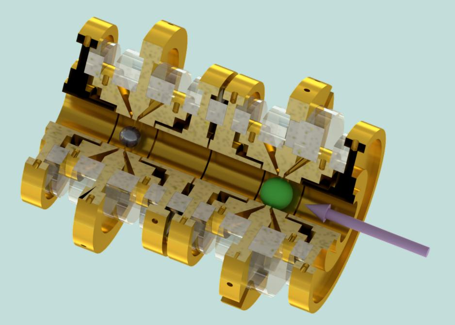
A cloud of Be ions (green) is laser cooled to the Doppler-limit temperature of several mK, and interacts with a single proton (grey) via the image charge induced on the common endcap electrode.
