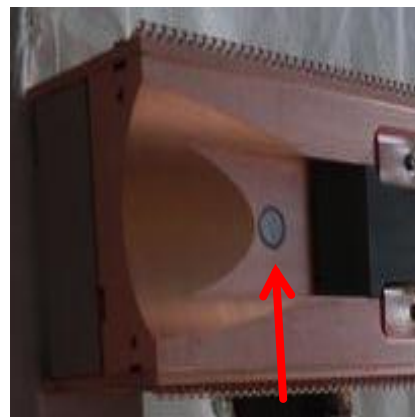
Equipped with BPM button on both end of the jaw (1m long)
