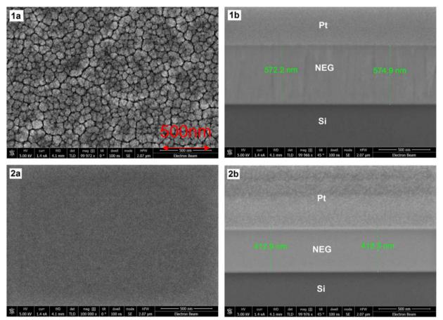
The high resolution (a) planar and (b) FIB prepared X-section SEM images of columnar (1a and 1b) and dense (2a and 2b) NEG films
