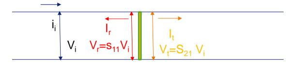
However, the resistance of the NEG coated kapton sheet resistance  $Z_s$  is easy to derive from the  $s_{11}$  reflexion and  $s_{21}$  transmission coefficients:
