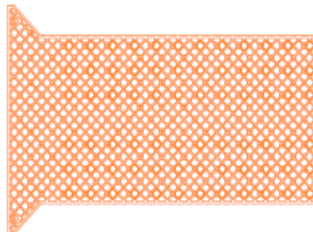
Polyimide meshed spacer (meshed area ~ 70%)
