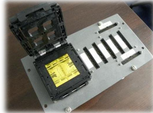
FoCal chipcables in test Socket (TAB-70)
