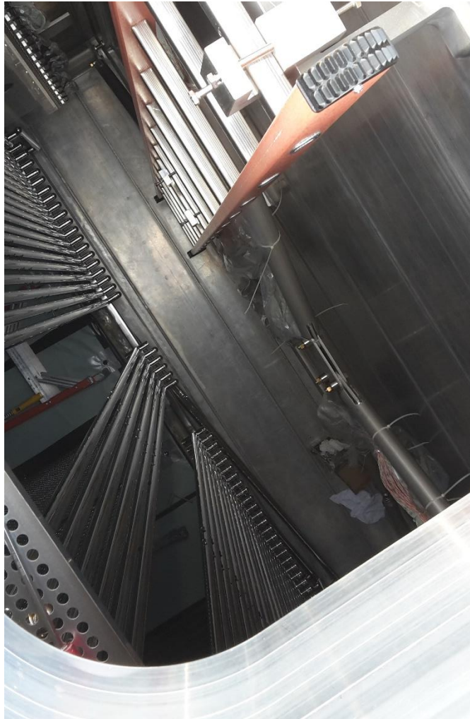
View from the man-hole of the race-tracks removed to access the drift volume.
