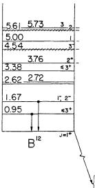
Excited states of <sup>12</sup>B are known! Comparison between the theoretical calculations (e.g. TALYS) and the available experimental data (e.g. Pillon et al.) as the basis for the estimation of the systematic uncertainties.
