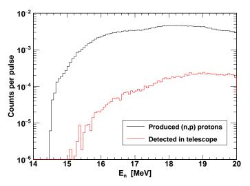
Detected counts reduced due to the limited solid angle, i.e. the geometrical efficiency (no ENDF data above 20 MeV).
