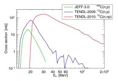
Above 25 MeV the proton yield from the  $^{12}C(n,np)$  reaction is expected to start mixing with the  $^{12}C(n,p)$  yield.
