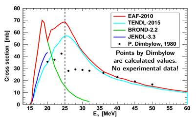
The peak of EAF-2010 for (n,d) at 70 mb, the same as TENDL-2009 for (n,p) [see previous slide]  $\Rightarrow$  similar statistics expected for both reactions.
