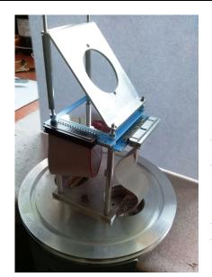
Intended use of the updated, geometrically optimized setup, comprising double the number of channels/Si-strips (64 in total) and featuring a very wide angular coverage  $(10^{\circ}-150^{\circ})$ .
