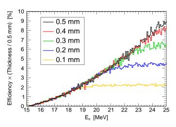
0.2--0.3 mm: the optimum between the detected reaction yield up to 25 MeV and the background induced by the secondary reactions.
