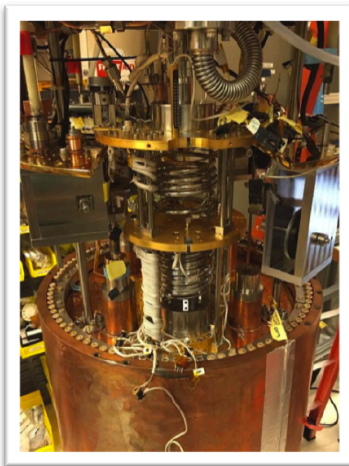
Dilution Refrigerator installed above ADMX Cavity
