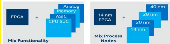
Figure 6. Heterogeneous In Package Integration with 3D SiP Technology
