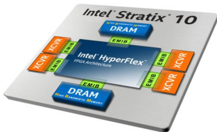
Figure 6. Heterogeneous In Package Integration with 3D SiP Technology
