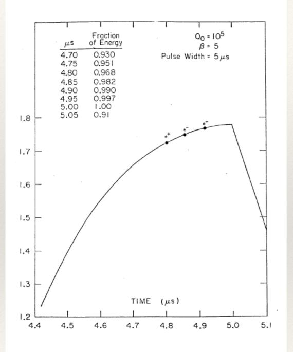
K. Oide suggests 4 bunches per RF pulse during e+ creation, yet arising the question of hitting/moving the positron target between e- e+ bunch spacing.
