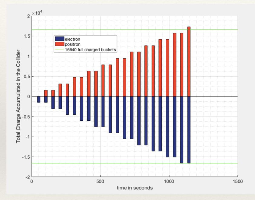
Notice that the e- and e+ charges are asymmetric, e+ buckets of collider has 104% while e- buckets are with 100%. To obtain that configuration, for example, we add 9.5% to the e+ at the last cycle.
