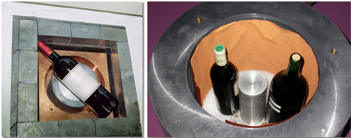
Fig. 4: \gamma -ray measurement. [left] Bottle laying flat on a Ge detector. [right] 2 bottles shown against the Germanium detector just for illustration purpose.
