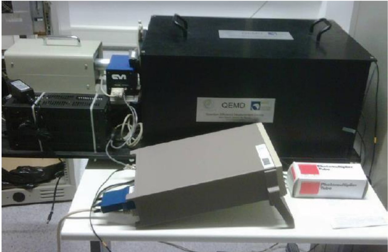
Fig.2. QE measuring custom-designed device in MPI. On left top one can see the light source (grey box) accommodating a deuterium and a halogen lamps, the small blue box is a modified spectrometer. Light from it enters into the sensor test dark box via a filter wheel. In front is shown a Keitley pico-Ammeter (grey) of type 6485.
