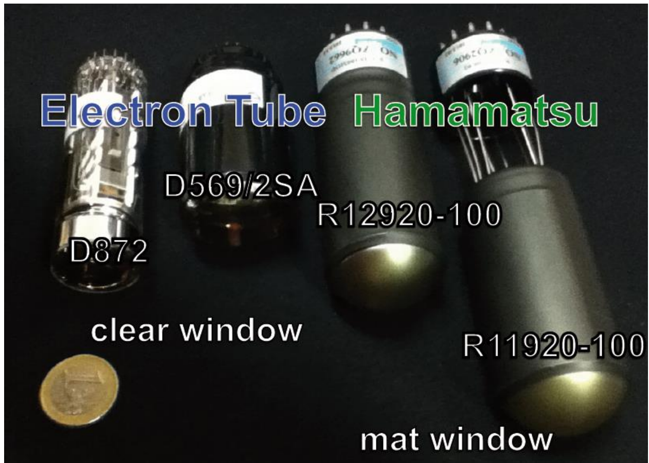
Fig.1. Photo of candidate PMTs for CTA. Left: prototype test-bench PMT D872 from ETE; 2 nd from left: 8-dynode PMT D569/2SA from ETE, 3 rd from left: 7-dynode (final) PMT R12920-100 from Hamamatsu; 4 th from left: 8-dynode PMT R11920-100 from Hamamatsu. Note that the PMTs from Hamamatsu have a mat input window.
