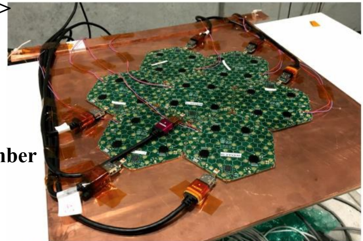
Figure 5.12: Seven 6" silicon sensor modules, equipped with SKIROC2-CMS ASIC, mounted on a copper support/cooling plane during the 2017 beamtest campaign.
