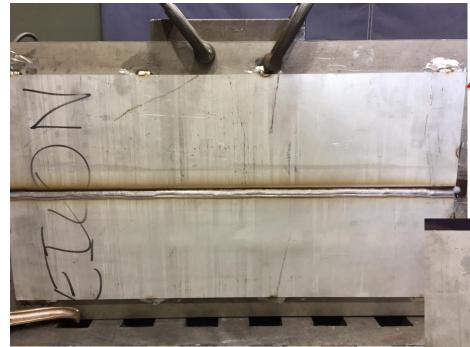
Root Pass – sample plates tacked to base prior to welding
