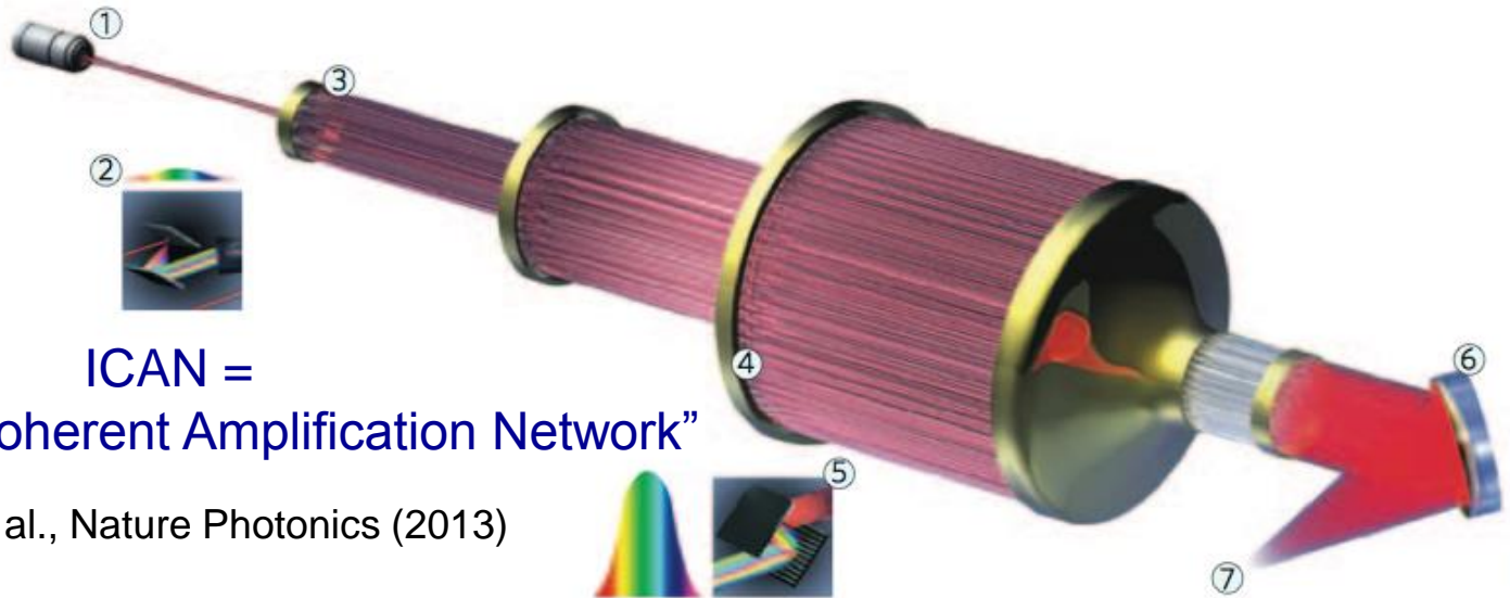
Figure 1 | Principle of a coherent amplifier network. An initial pulse from a seed laser (1) is stretched (2), and split into many fibre channels (3). Each channel is amplified in several stages, with the final stages producing pulses of ~1 mJ at a high repetition rate (4). All the channels are combined coherently, compressed (5) and focused (6) to produce a pulse with an energy of >10 J at a repetition rate of ~10 kHz (7).
