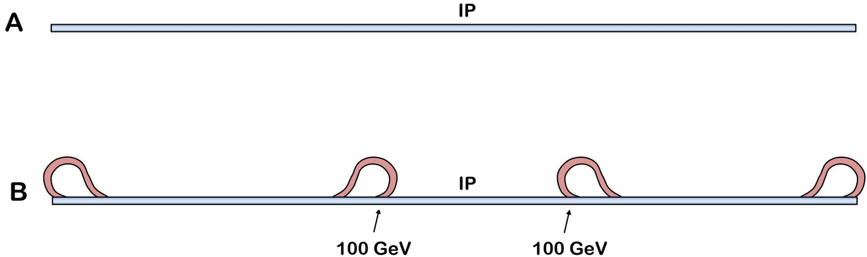
**Possible Civil Construction provisions for 250 GeV ILC Higgs factory tunnel layout that enable 1-2 TeV CM upgrade in the future (if this concept will be proven viable).**
