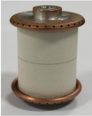
Fig. 7. Implementation of the scaling methods described herein have resulted in a device which has withstood 13,000 pulses of 250-265 kV, without encapsulation. The tested device shows promise for a corresponding 500 kV device with twice the thickness and encapsulation.
