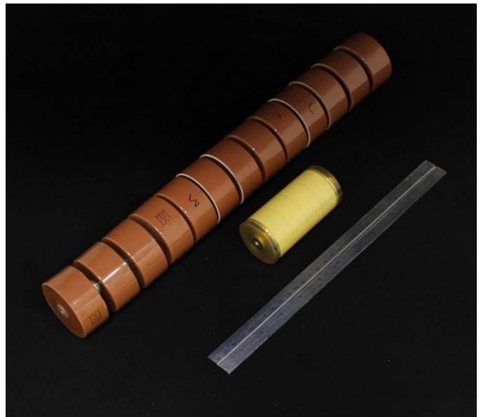
Fig. 5. An encapsulated 500 kV capacitor prototype is shown next to a 500 kV assembly of TDK door knob capacitors along with a ruler for size reference. The capacitor development effort has resulted in 500 kV capacitors that fit in the palm of the hand.
