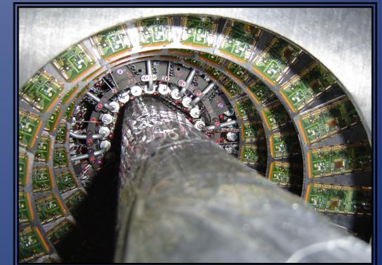
Add a new b-layer around a smaller beam pipe (in radius), stave structure, 160 MHz readout, CO<sub>2</sub> cooling
