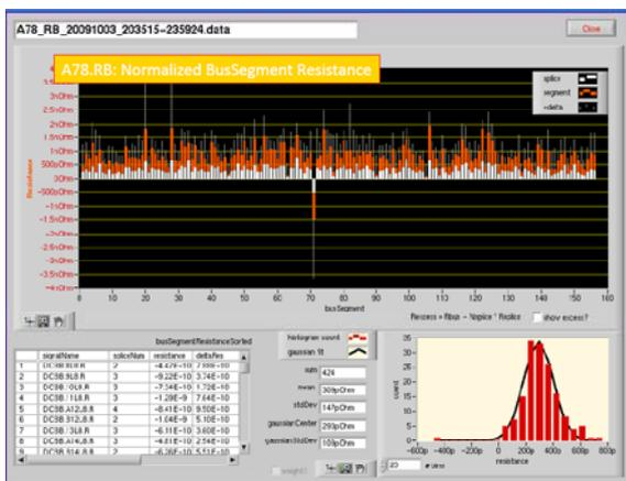
Figure 1: Splice resistance measurement in sector 7-8.
