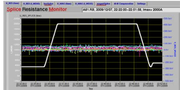
Figure 2: Resistive voltage during ramp and coasting after fine tuning of the inductive compensation values in sector 8-1.
