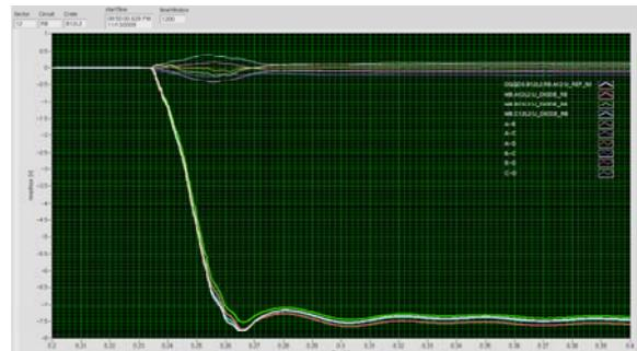
Figure 3: Activation of energy extraction systems at  $I = 4$  kA in sector 1-2 and data recorded by a symmetric quench detection board (dump of diagnostic buffer).
