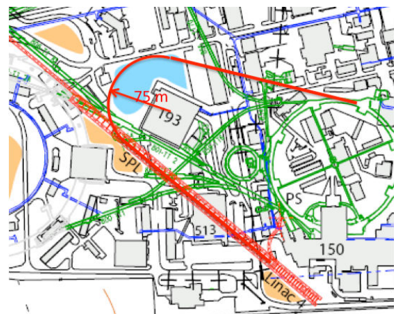
Figure 3: Possible geometry of a 2.5 GeV SPL injecting into the PS.
