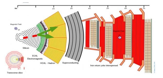
Decay in the tracker : Displaced track signature No missing transverse energy
