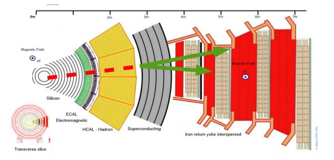
Decay in the Calorimeters : Calorimeter/Muon signature Missing transverse energy
