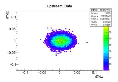
Field off scattering analysis uses a 200ps width TOF01 cut to segment momentum.
