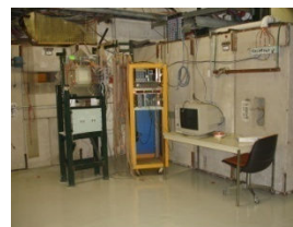
4 station MWPC spectrometer
