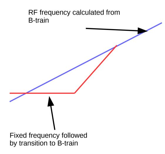
\*N.B.: Bdl and Fixed frequency line lengths are the same here because I'm lazy, no inherent connection between the two in the machine
