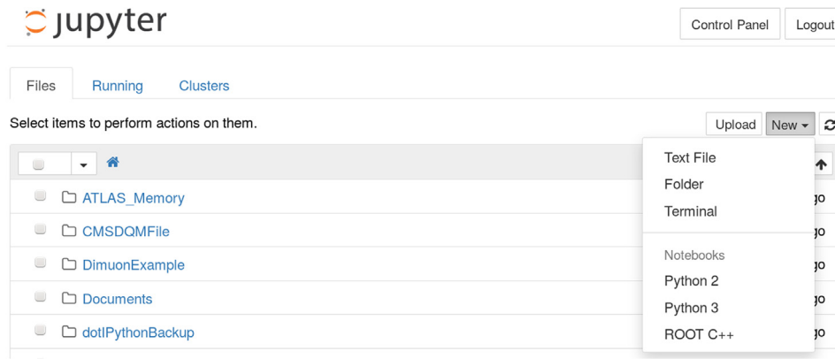
Fig. 3. The web interface of the Jupyter server. The content of the home directory is displayed. The drop-down menu shows that it is possible to create a text file, a directory or open a terminal. Different notebook flavours can be seen too. In this example Python2, Python3 and C++ languages are available. The interface also allows to upload files.
