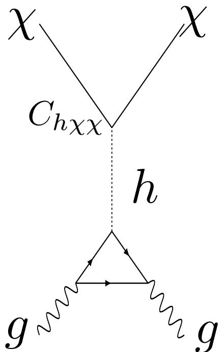
$$f_N/M_N = -\frac{C_{h\chi\chi}}{vm_h^2} \left[ \sum_{q=u,d,s} f_{Tq}^N + \frac{2}{9} f_{TG}^N \right]$$
